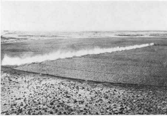
Photo 2: A center pivot system in operation in central Washington's Grant County. Note the more expansive discharges of water near the outer end of the lateral than near the pivot point (Courtesy of Valmont Industries, Inc.)
