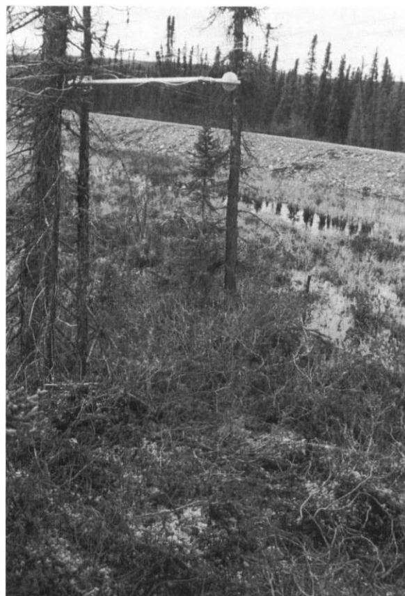
Photo 1: The Q-6 Net Radiometer mounted 1.5 m above a typical example of the dominant vegetation cover on the peat plateau at km 161.7, Robert Campbell Highway, Tuchtua
