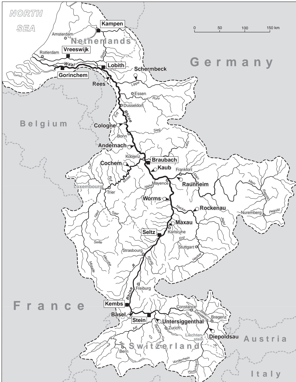
Fig. 1: The River Rhine basin with catchment borders of main tributaries and interim basins. Gauges for description of hydrological regimes and biogeochemical fluxes are depicted
