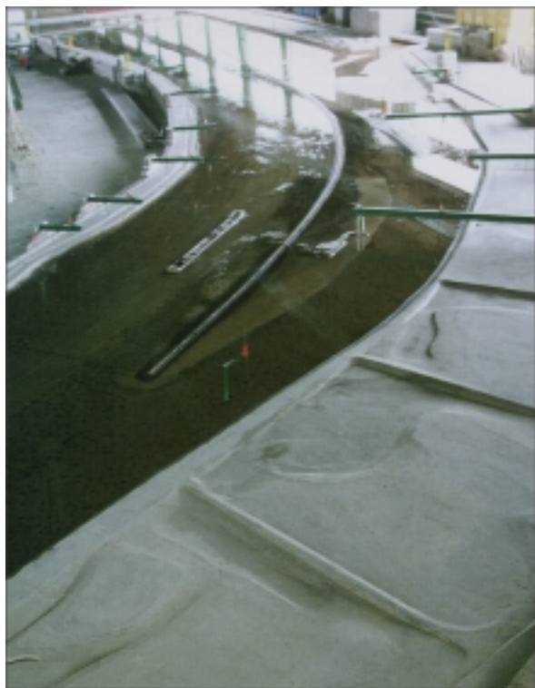
Photo 3: Model of the “Binger Loch” for tests of the hydraulic consequences of further measures
