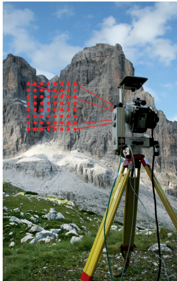
Photo 3: The Riegl LPM-321 terrestrial laser scanner stationed in front of Rifugio Brentèi (2182 m) while scanning the famous Cima Tosa (3146 m) Ice Couloir
