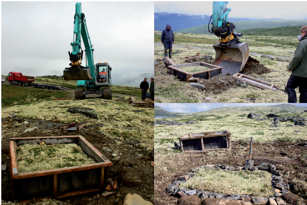
Fig. 4: Transplantation of 1.5 \times 1.5 \times 0.5 \text{ m}^3 monoliths to a lower altitude (Vägå/Oppland, Norway, summer 2008)
