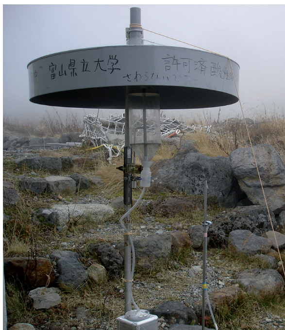
Photo 2: Passive thin-string fog water sampler mounted at Murododaira
