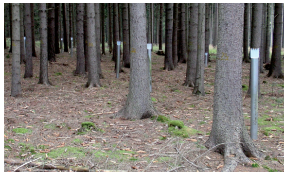
Fig. 3: Throughfall sampling, site Košetice
