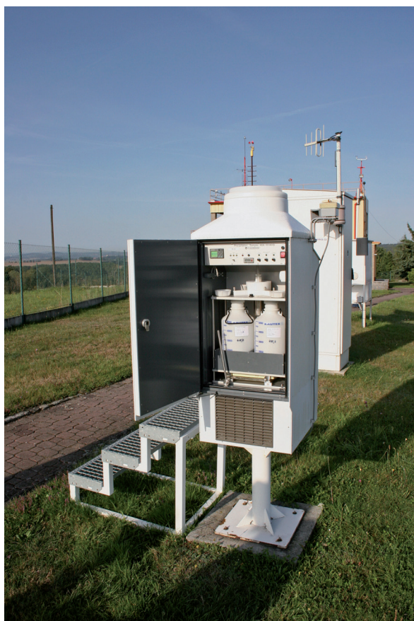
Fig. 2: Wet-only sampler, site Kocelovice
