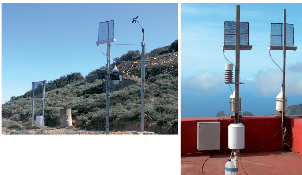
Photo 3: The equipment used in the stations at Boutmezguida is a SFC and a QFC (photo on the left) and Anaga there are two QFCs with different meshes (photo on the right). In both cases the meshes are connected to meteorological stations (© Marzol)
