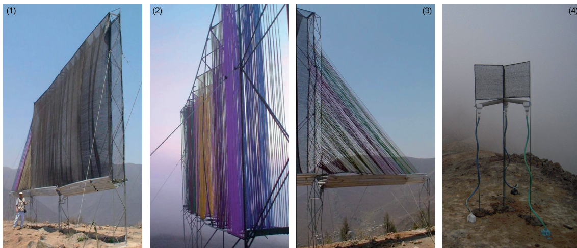
Fig. 1: Compared full scale fog water collection devices as developed from the design study (see also Tab. 1): (1) “Eiffel” collector – 4x8x0.3 m metal frame, two separated layers of Raschel 50% net with 10 additional stripes in between; (2) “Harp” collector – 2x4x0.3 m metal frame, 2,256 m of 1.5 mm rubber string vertically installed; (3) “Diagonal Harp” collector – 2x4x0.3 m metal frame, 1,520 m of 1.5 mm rubber string diagonally installed; (4) The Astropod screener with star-shaped screening wings
