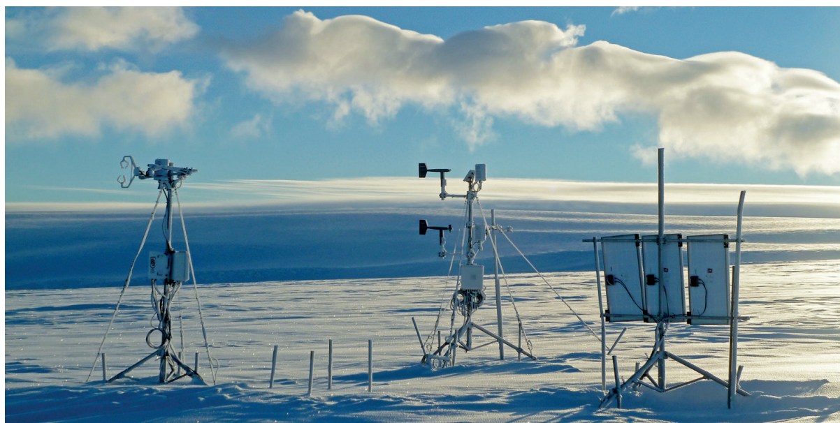
Photo 2: Automatic Weather Station (AWS) during the accumulation period on the Fourcade Glacier. (Photo: D. LÓPEZ 2012)
