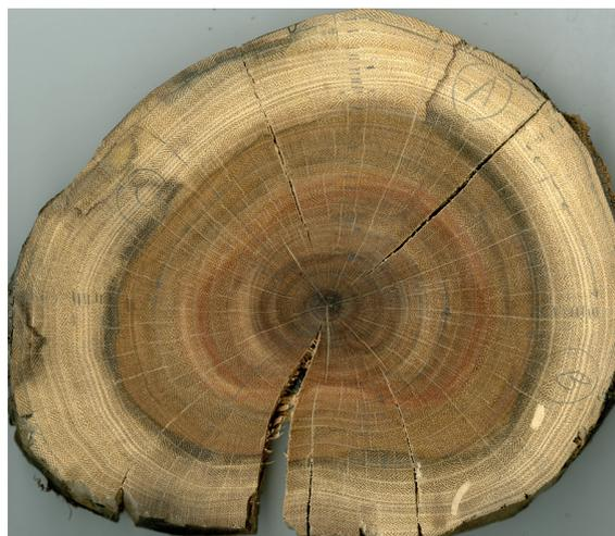
Photo 3: Stem disk of Māmane (diameter ca. 18.5 cm). Tree rings, as well as sap wood and heart wood boundaries are easy to distinguish.
