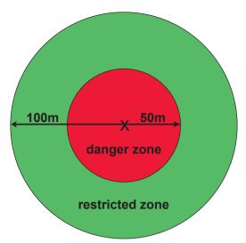
Fig. 1: Schematic depiction of position and minimum size of 'danger zone' and 'restricted zone' relative to the source of danger in the center (draft based on AFKZV 2012, 28; my translation).
